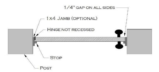
We also prefer to swing the doors to the inside to help protect the door from the rain. If you do swing to the outside, we add an aluminum cap over the door.
